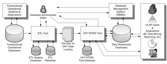
Figure 5. The 24/7 real-time data warehouse architecture.
