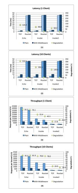
Figure 5. Latency and Throughput Degradation Caused by Middleware
