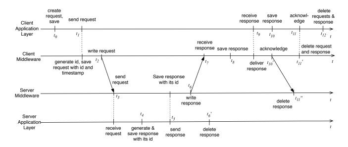
Figure 2. Exactly-Once Request-Response Pattern With Middleware Layer
