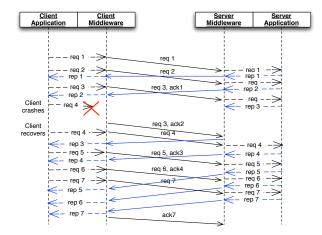
Figure 4. Recovery From Client Failure
