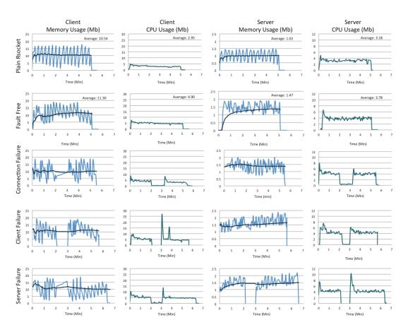
Figure 7. Memory and CPU usage with Middleware and RSocket under Connection, Client and Server Failure
