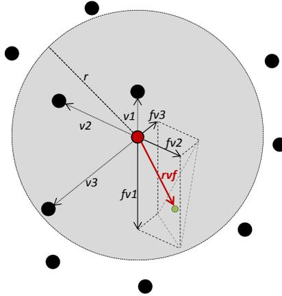
Fig. 1: Example of a Resultant Force Vector  $rfv$
