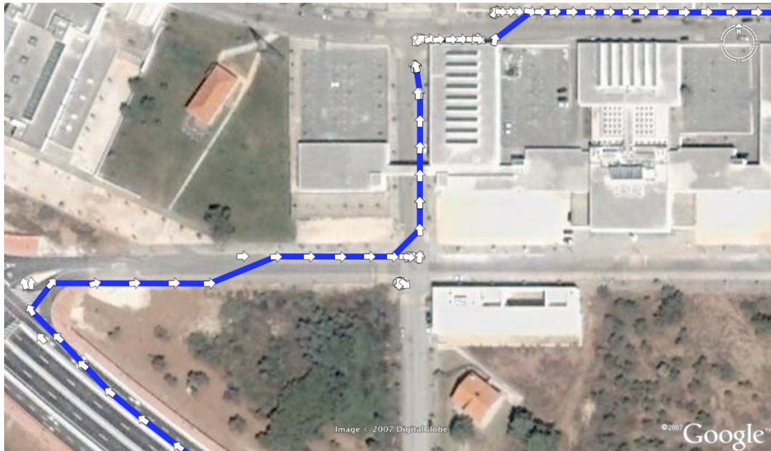
Figure 3 – Filter application to a GPS trace. The arrows indicate trace points, while the thick line corresponds to the filtered path proposed.
