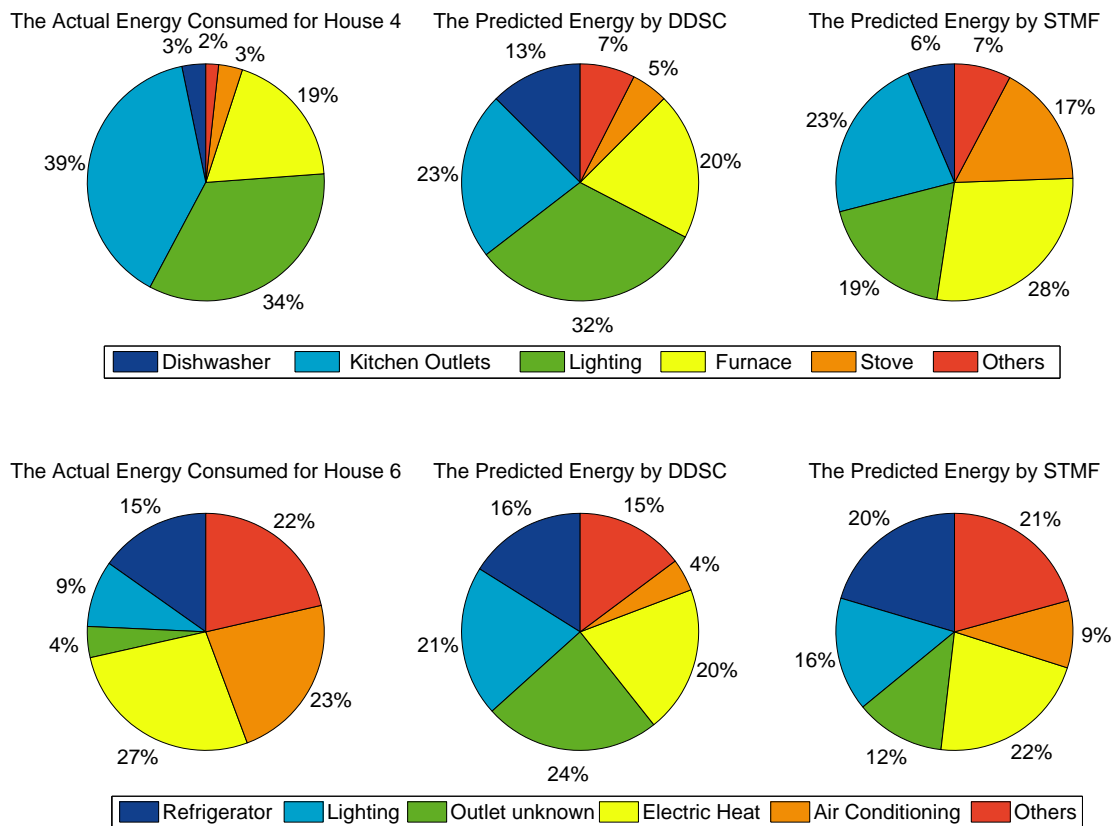
Figure 5.9.: Consumed and predicted energy by DDSC and STMF approaches for Houses 4 and 6.
