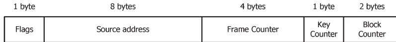
Fig. 4. Format of the Initialization Vector for AES-CRT and AES-CCM security in IEEE 802.15.4.
