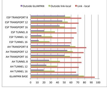
Figure 6. Payload space available with 6LoWPAN security without mesh or fragmentation headers
