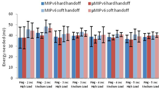
Figure 11. Average energy needed on each mobility request in Figure 3.
