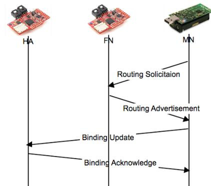
Figure 1. Mobile request in detail.
