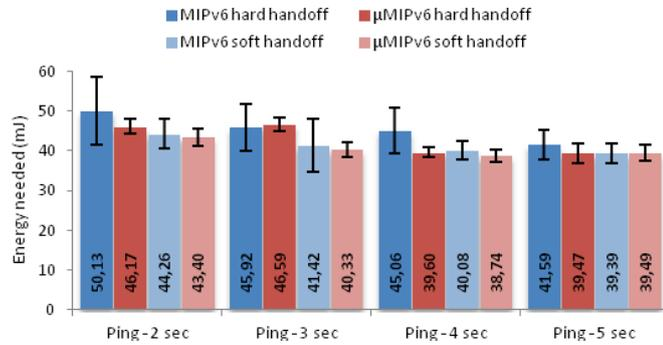
**Figure 7.** Average energy needed on each mobility request in Figure 2.
