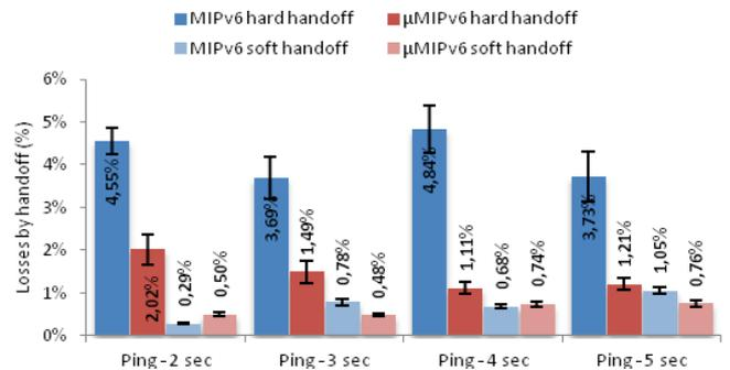
Figure 5. Percentage of ping losses by handoff in Figure 2.
