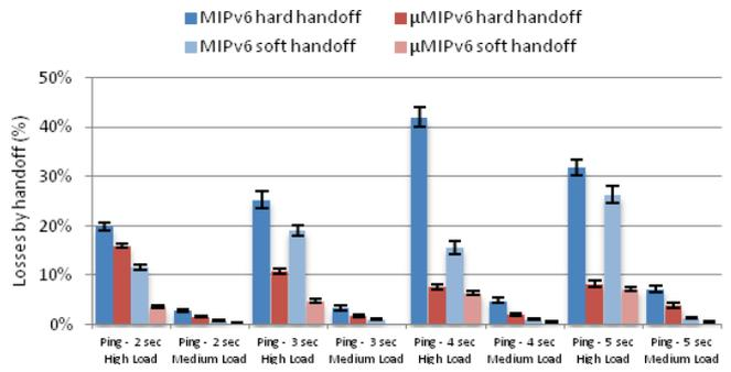
**Figure 9.** Percentage of ping losses by handoff in Figure 3.
