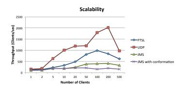
Fig. 5. Scalability of FTSL in comparison to JMS and UDP multicast
