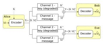
Fig. 1. Wiretap channel variant where an interleaving key K is sent with the original message M. The key is sent during a period in which a jammer is active, hence the degraded channels during the transmission of the key.
