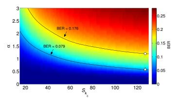
Fig. 3. BER on the interleaving key portion of  $[K_c \text{ inter}(M)]$  as function of varying jamming power  $P_j = \alpha P_a$  and key size  $S_{k_c}$ , for  $C_i$  an LDPC(1056, 880) code that provides a BER =  $10^{-5}$  for decoding a transmission over an AWGN channel at SNR = 6.38 dB. For B&W visualization, the gradient on the right bar follows the same order as in the plot.
