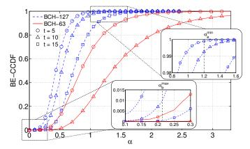
Fig. 4. BE-CCDF of  $K_c$  as a function of a jamming power of  $P_j = \alpha P_a$  applied over  $K_c$ , for  $C_i$  an LDPC(1056, 880) decoding at the selected SNR of 6.38 dB for reliability. We consider two key sizes  $\mathcal{S}_{k_c} = [127, 63]$  that relate to BCH codes of those lengths ( $\mathcal{S}_{k_c} = \eta_o$ ). The different markers correspond to the number of errors t = [5, 10, 15] that the BCH codes (127, [92, 64, 36]) and (63, [36, 18]) can correct.
