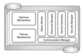
Fig. 2: Hybrid Orchestrator Architecture
