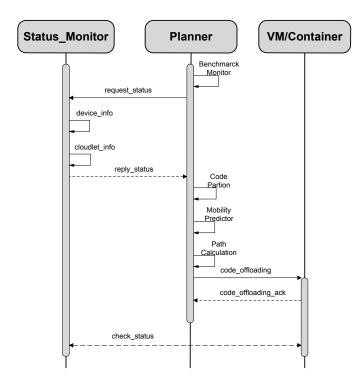
Fig. 4: Sequence Diagram: Code Offloading in a Mobility Scenario
