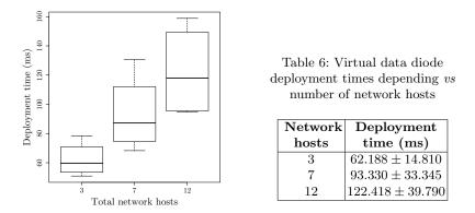
Fig. 8: Virtual data diode deployment times *vs* number of network hosts.
