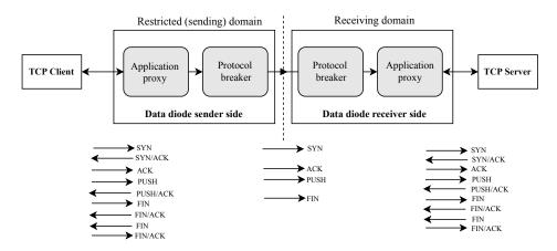
Fig. 1: TCP workflow in uni-directional gateways (adapted from [6]).
