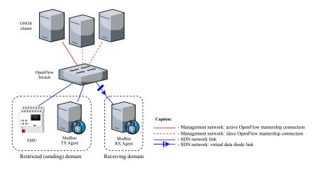
Fig. 5: Experimental testbed.
