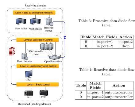
Fig. 2: SDN-enabled virtual data diode.
