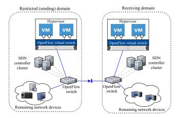
Fig. 3: NFV assisted SDN virtual data diode.
