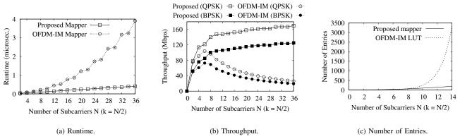
Fig. 2. Proposed mapper vs. OFDM-IM index selector mapper under the maximal spectral efficiency: runtime (a), throughput (b) and number of table entries compared to the LUT-based OFDM-IM mapper (c).
