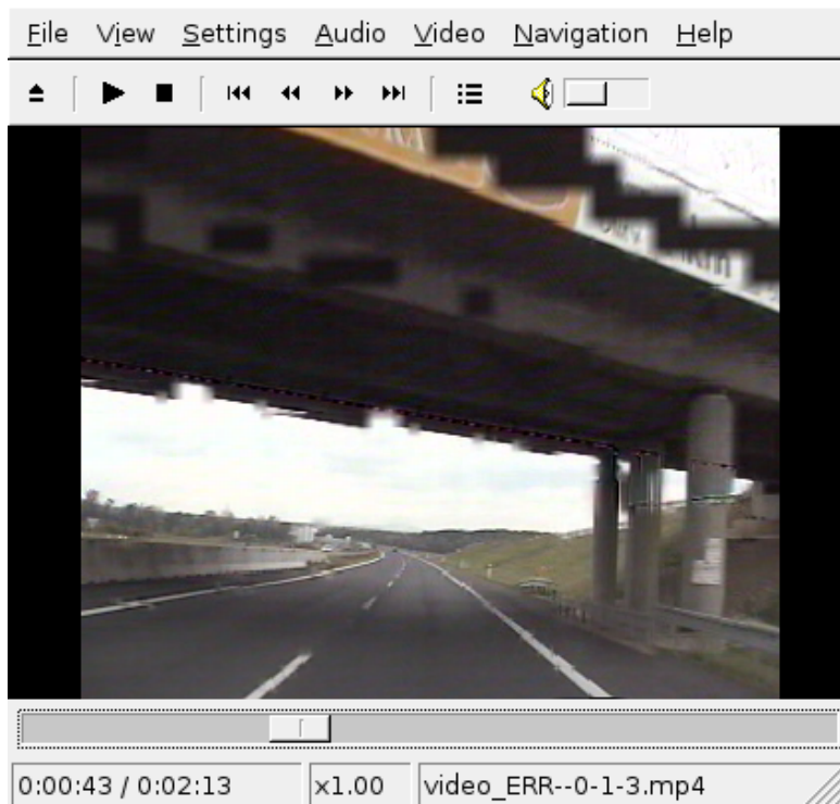
Figure 5.11: Image of the video transmitted in a Link Going Down test case
