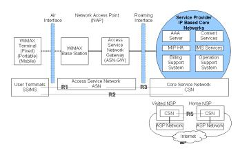
Figure 1: WiMAX Network Architecture
