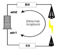
Figure 3 - Test-bed for voice and video evaluation
