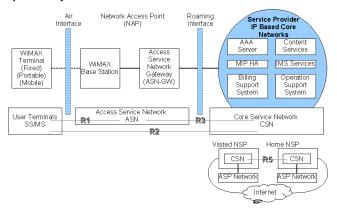
Figure 2 - WiMAX network architecture
