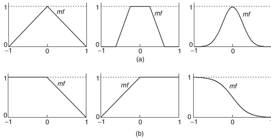
**FIGURE 4.9** Membership functions: (a) symmetrical (triangular, trapezoidal, Gaussian); (b) nonsymmetrical.
