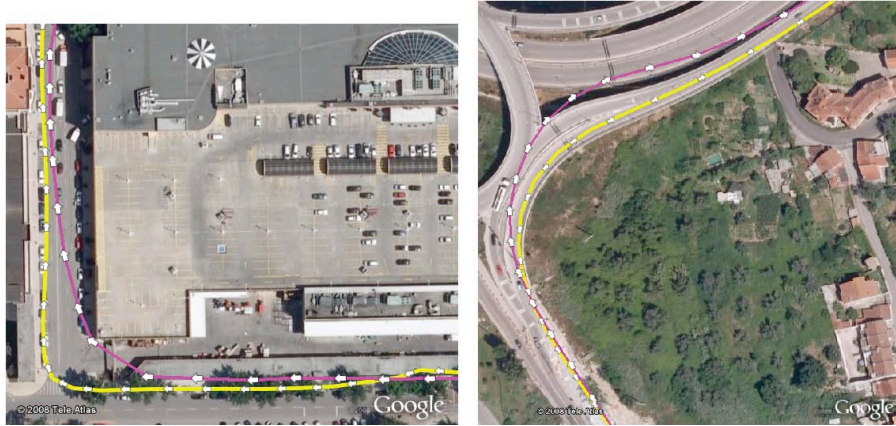
Figures 5 and 6 – Difference between map and trace patterns in curves. The yellow line represents the map and magenta the trace.
