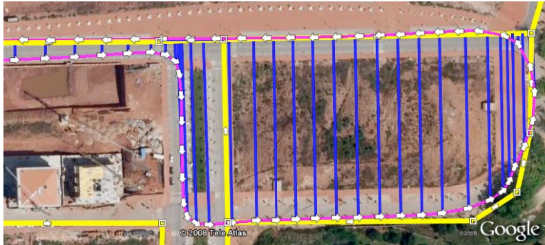
Figure 11 – Marchal’s original algorithm: Given the absence of a descending road in the center, the algorithm insists on keeping the match to the upper road 4 .
