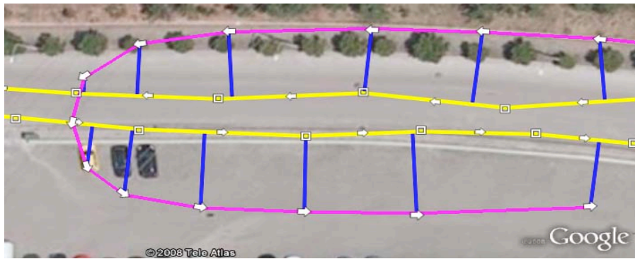
Figure 19 – GEMMA: The same scenario as in Fig. 17. The U-turn with the Genetic Algorithm
