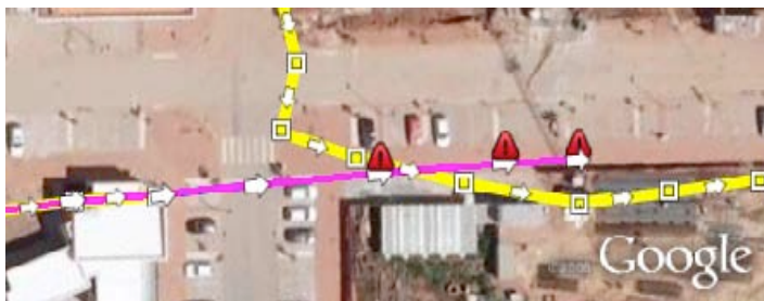
Figure 18 – Small matches being ignored by Marchal Based Algorithm.
