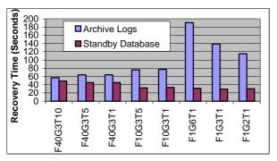
Figure 9. Standby database recovery time vs recovery time with archive logs.
