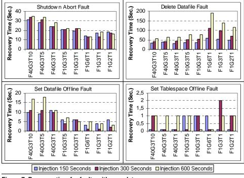
Figure 7. Recovery time for faults with complete recovery.
