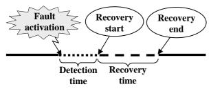
Figure 2. Steps in the injection of an operator fault.
