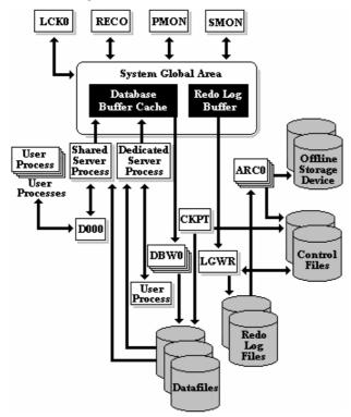
Figure 1. The Oracle 8*i* background processes and recovery structures [15].
