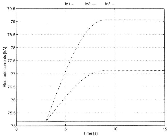
Figure 5.32 The electrode currents when lowering electrode 3
