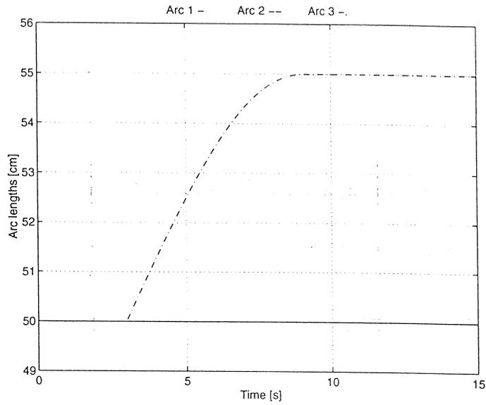
Figure 5.33 The arc lengths when lifting electrode 3
