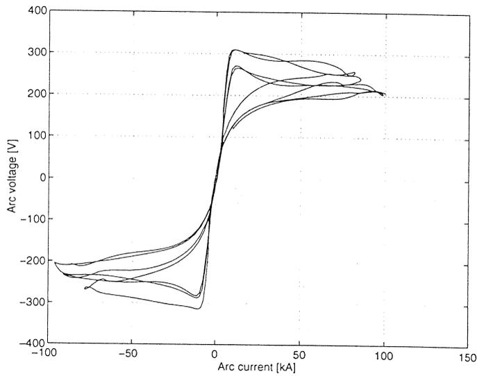
Figure 5.16 The dynamic arc current-voltage characteristic after 7 minutes
