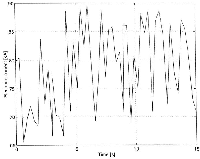
Figure 5.36 The effect of disturbances in the electrode currents
