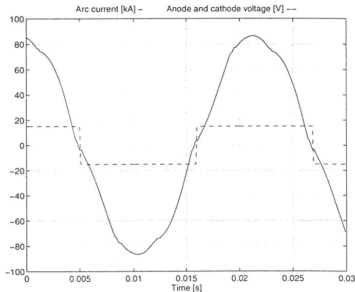
Figure 5.6 The anode and cathode voltage delay
