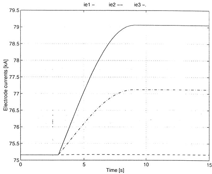
Figure 6.6 The electrode currents when lowering electrode 1
