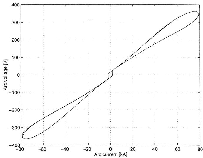
Figure 5.20 The dynamic arc current-voltage characteristic after 27 minutes
