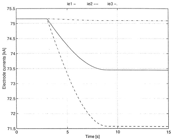
Figure 5.30 The electrode currents when lifting electrode 2
