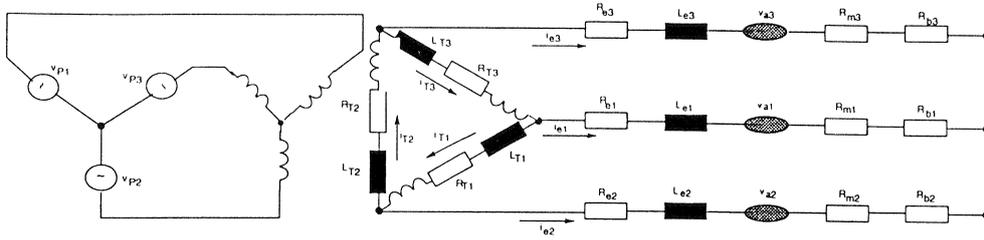
Figure 4.2 The equivalent circuit of the EAF
