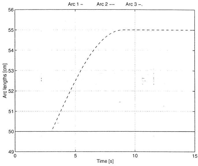
Figure 5.29 The arc lengths when lifting electrode 2
