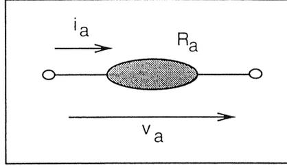
Figure 3.9 The electrical arc as a circuit element
