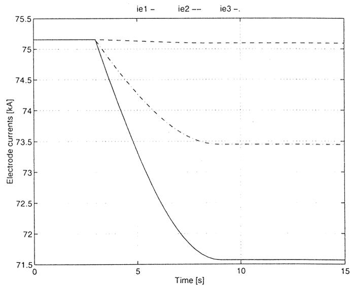
Figure 5.26 The electrode currents when lifting electrode 1
