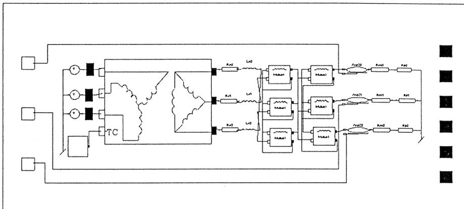
Figure 5.22 The EAF diagram for the steady-state model
