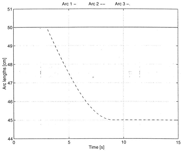
Figure 5.27 The arc lengths when lowering electrode 2
