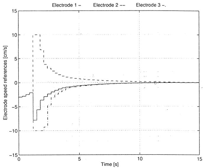
Figure 6.9 The control signals for a step disturbance
