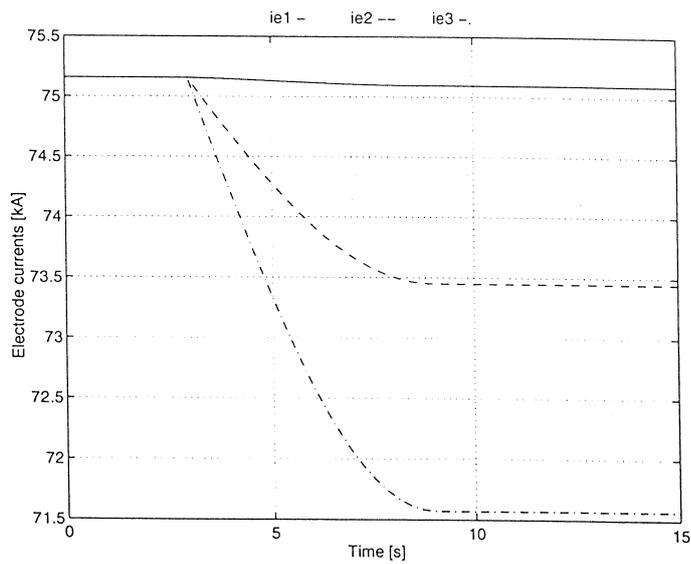
Figure 5.34 The electrode currents when lifting electrode 3
