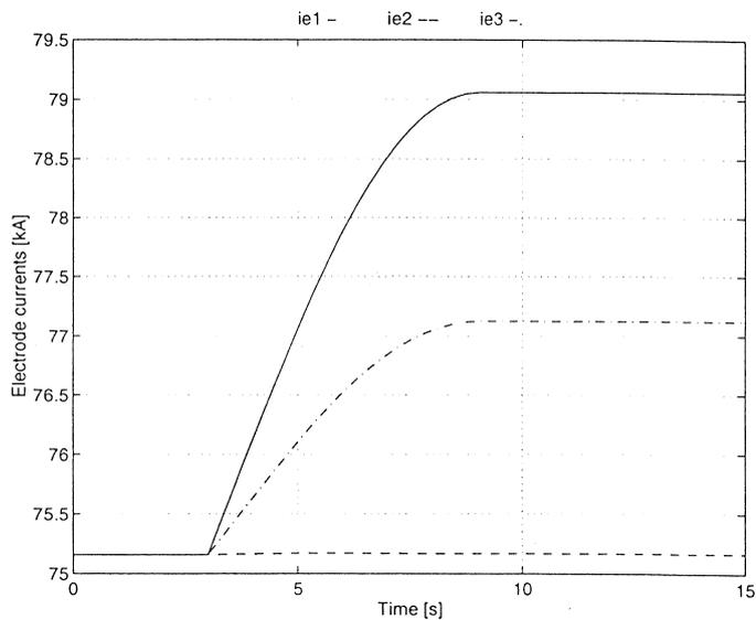
Figure 5.24 The electrode currents when lowering electrode 1
