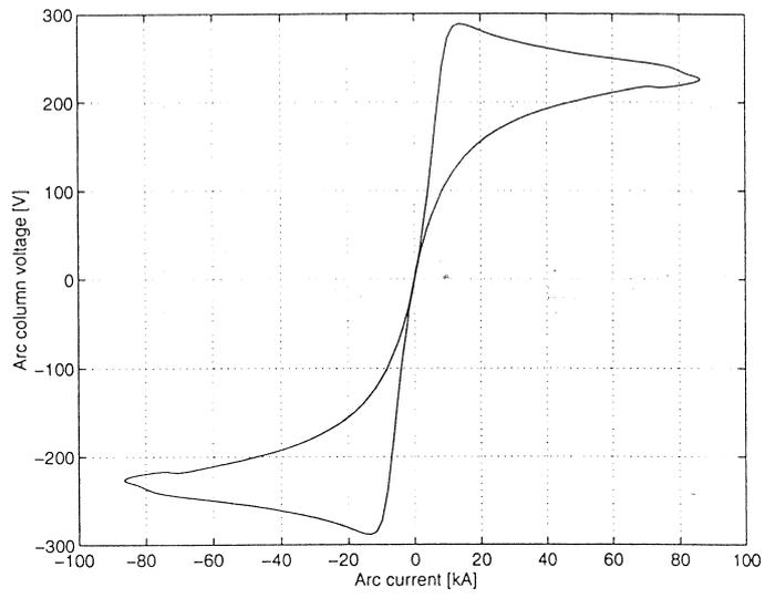
Figure 5.3 The dynamic arc column current-voltage characteristic
