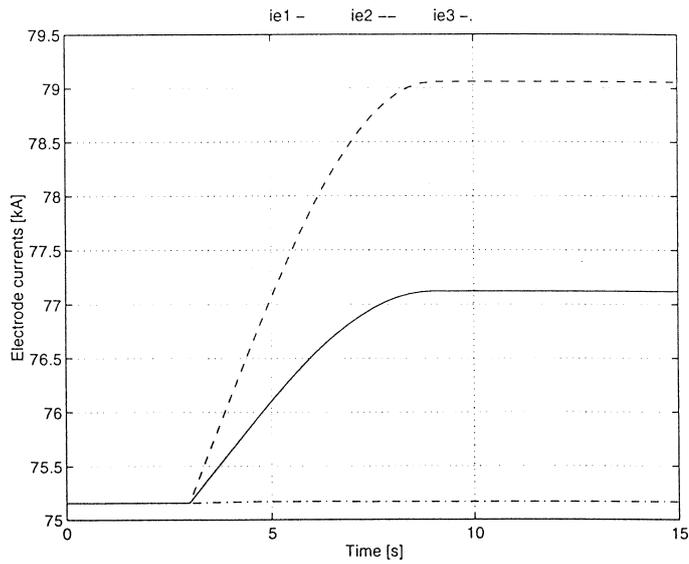
Figure 5.28 The electrode currents when lowering electrode 2
