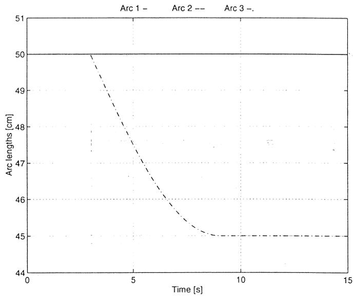
Figure 5.31 The arc lengths when lowering electrode 3
