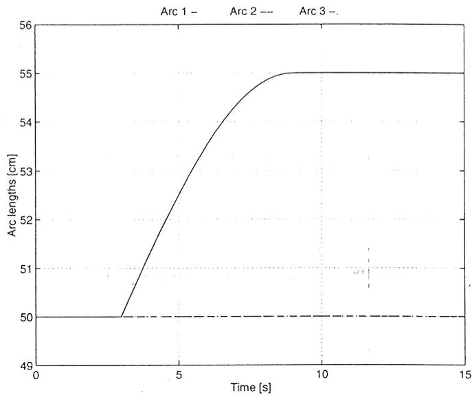
Figure 5.25 The arc lengths when lifting electrode 1
