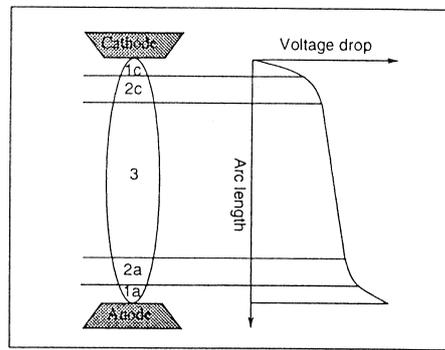
Figure 3.1 The potential distribution in an electric arc
