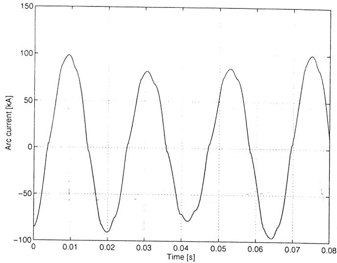
Figure 5.15 The arc currents after 7 minutes
