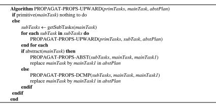
Fig. 9. Recursive algorithm for propagating properties upward, from primitive tasks to all non-primitive tasks
